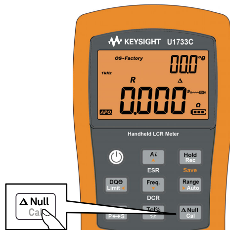
Figure 2-18 Using the Null function
