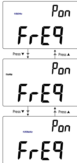
Figure 3-2 Changing the power-on test frequency
