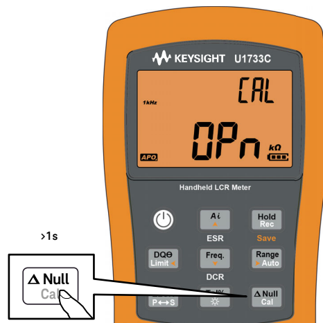
Figure 2-19 Using the Cal function
