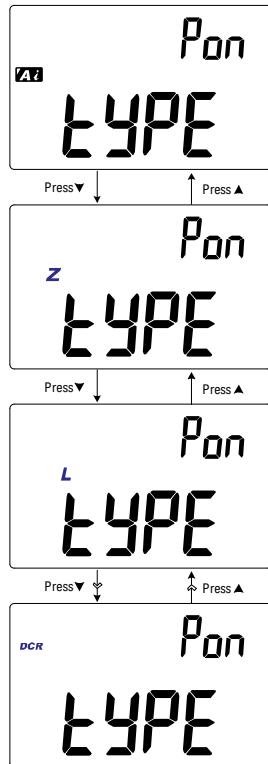
Figure 3-1 Changing the power-on measurement type
